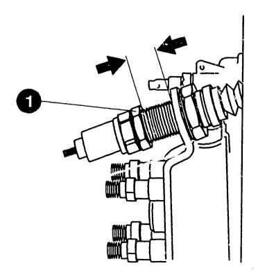
ADJUSTING TEMPERATURE—DEPENDENT IDLE INCREASE ACTING ON HOUSING—FIXED IDLE SPRING
